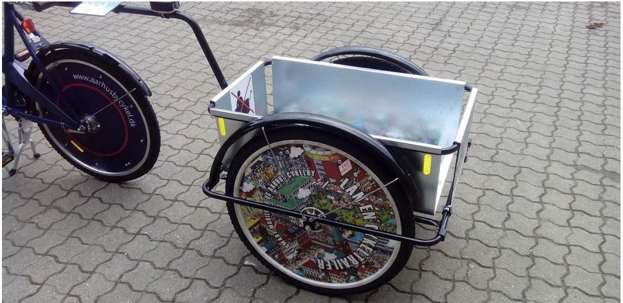
The trailers can carry up to 50 kilograms and can only be used for cargo.
