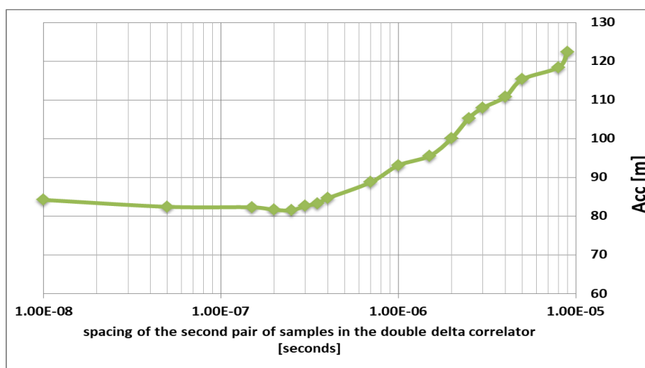
Figure 6-23: The accuracy of the distance as a function of the spacing of the pair of samples in the correlator
