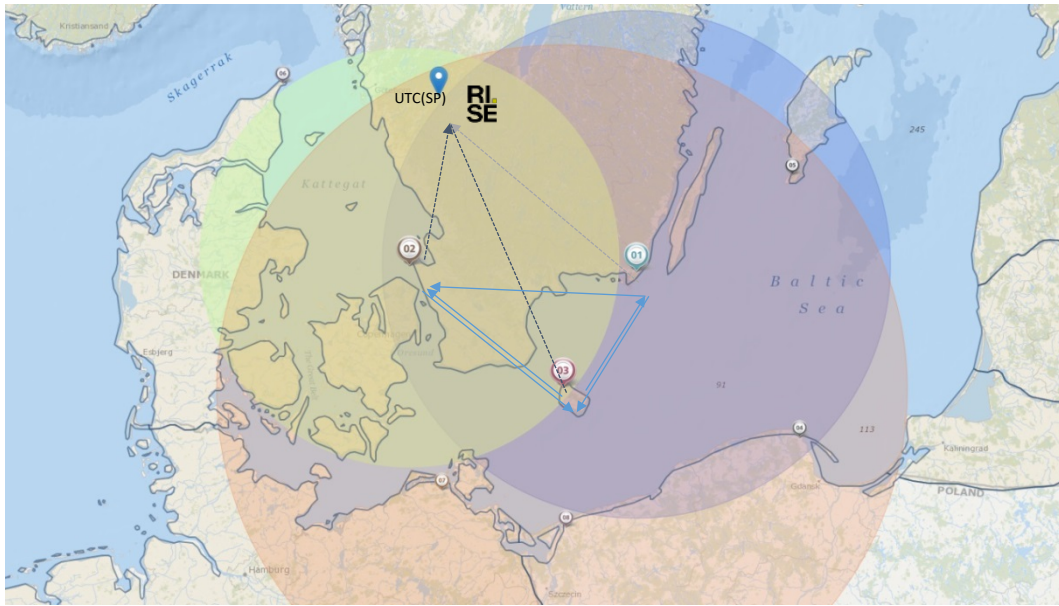
Figure 4 - Overlapping of signal reception can be used to form a self-sustained R-Mode synchronisation network of R-Mode stations. Map created using https://mapmaker.nationalgeographic.org/
