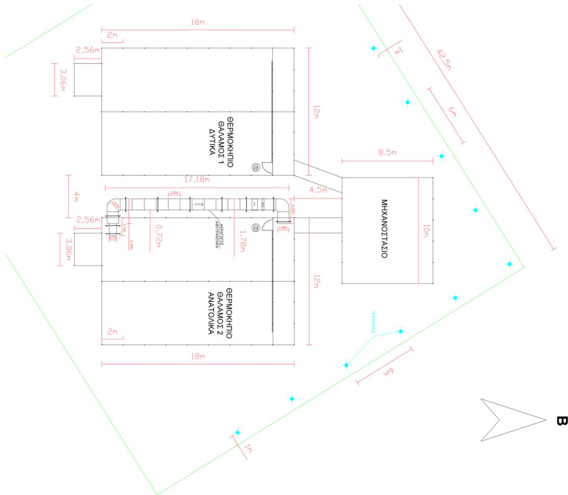
**Figure 1**– Top view of the MED Greenhouse installed in Larissa, including the geothermal boreholes
