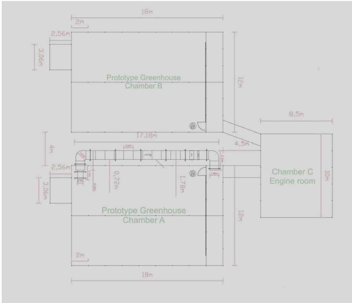
Figure 7– Top view of the MED Greenhouse in Larissa
