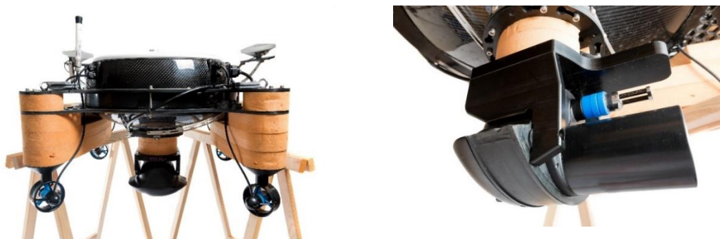
Fig. 3 Autonomous surface vehicle PlaDyBath with Trimble GPS antennas in the back and WiFi antenna on the left (left), close-up of the mounted multibeam sonar (right).
