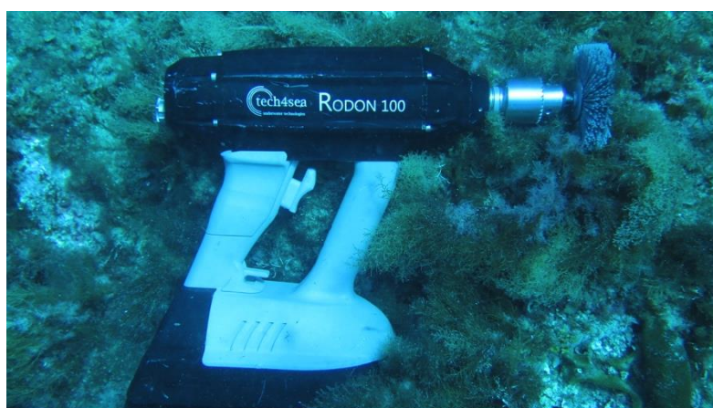
Fig. 5: Underwater drill Rodon 100, Tech4sea patented system.
