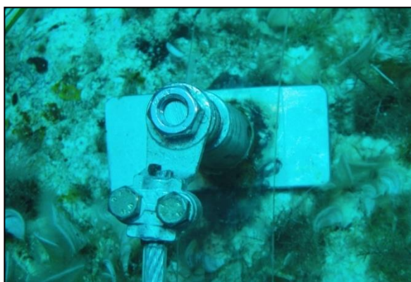
Fig. 2: Photographs of the new system for connecting the anodes to the cannons; a) detail of the tip placed under the graphitization layer and b) the Melinex strip.
