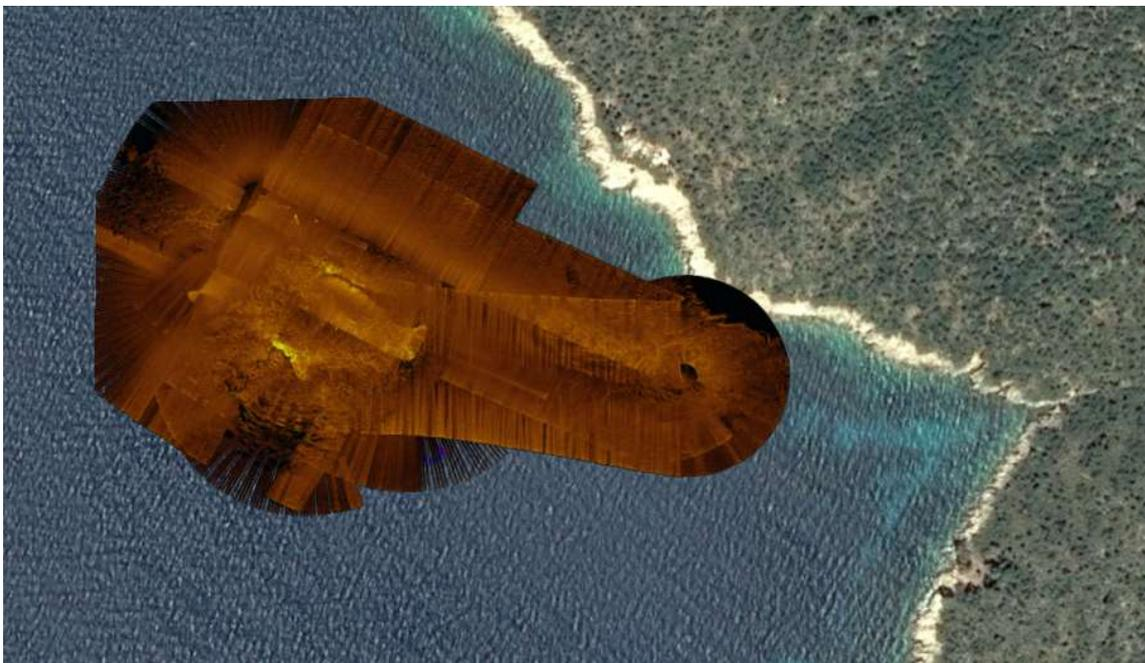
Figure 20. Side-scan sonar mosaic of the Peristera site georeferenced and shown in Google Earth
