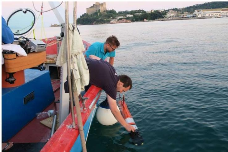
Figure 7. Deployment of the AUV for side-scan sonar survey mission
