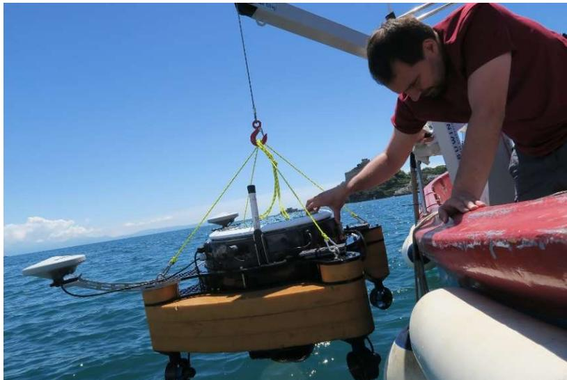
Figure 3. Deployment of the ASV by a transportable crane.
