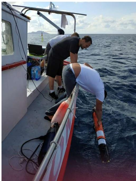
Figure 18. AUV Lupis deployment from the side of the boat
