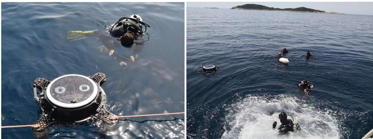
Figure 12. In-sea testing of the integrated SBL diver localization system (left). SBL ASV in dynamic positioning mode at the reference buoy position for the divers (right).
