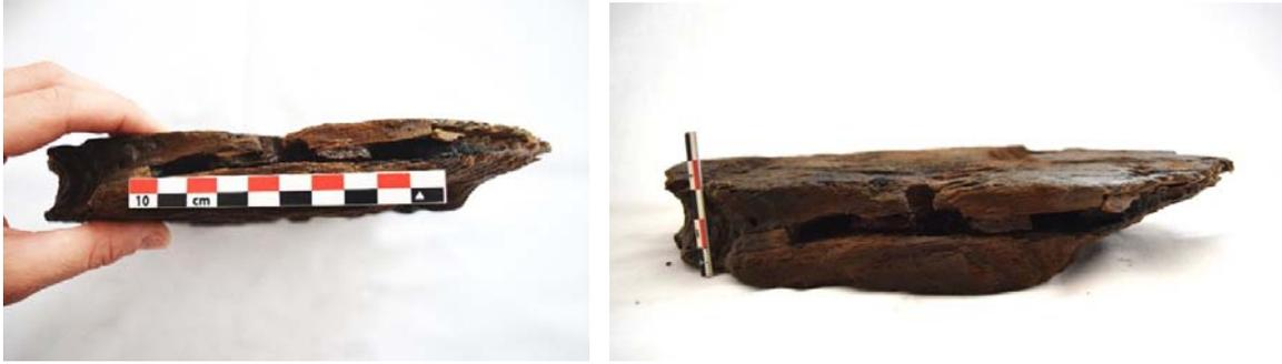
Fig. 12, 13 The remains of ship's planking with the mortise and tenon joinery
