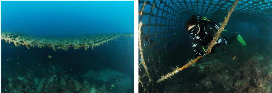
Fig. 7, 8 Degradation of the iron cage after two decades (photos: M. Brzac)
