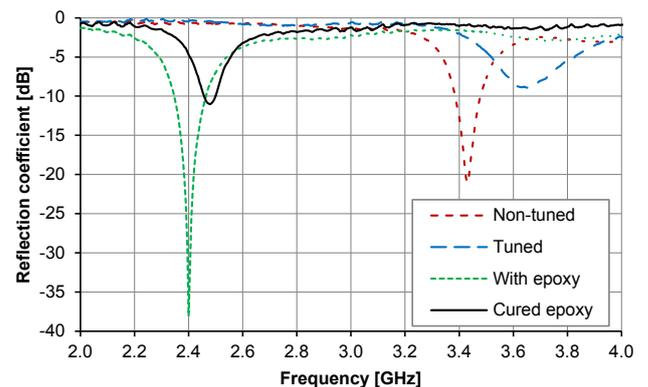
Fig. 2. Antenna reflection coefficient tuning.
