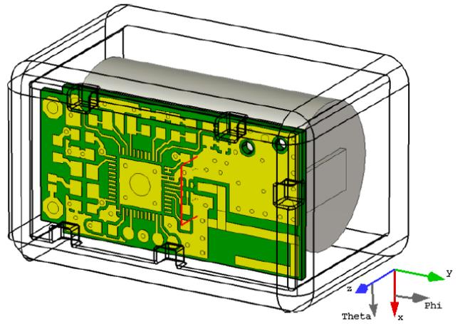
Fig. 1. Tag 3D model for antenna simulations.
