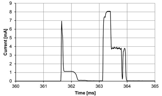
Fig. 9. Current consumption of the tag during the beacon transmission.
