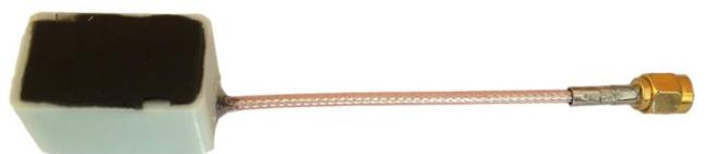
Fig. 3. Modified tag with external connection for antenna measurement.
