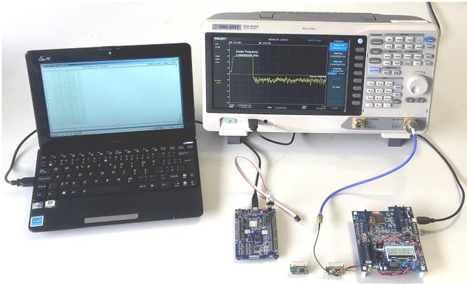
Fig. 7. ANT testbed: tag prototypes, nRF51-DK, X-NUCLEO-LPM01A, spectrum analyzer, and a laptop.
