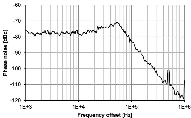
Fig. 8. Phase noise of a CW transmission at 2.44 GHz with 0 dBm power.
