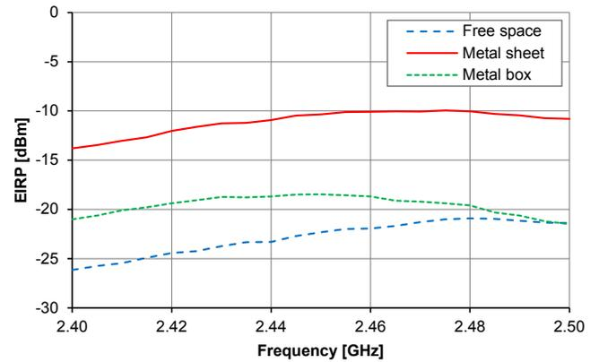
Fig. 6. Measured EIRP in z-direction of the tag placed in free space (long dashed), on a metal sheet (solid), and in an open metal box (short dashed).
