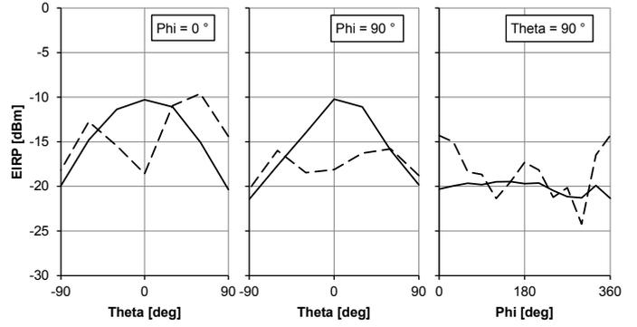
Fig. 5. Measured radiation pattern of the tag placed on a metal sheet (solid) and in an open metal box (dashed).
