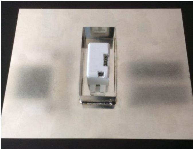
Fig. 4. Tag inside an open metal box.
