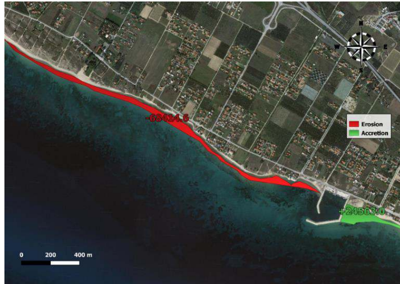
Figure 1. The coastal erosion (in red color) and deposition (green color) along the coastal zone of Kariani.
