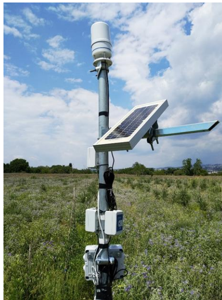
Figure 2 Meteorological station for IoT based irrigation system - Young olive grove
