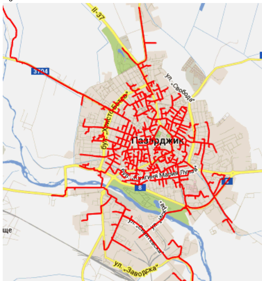
Figure 2.2: Gas distribution network in Pazardzhik
