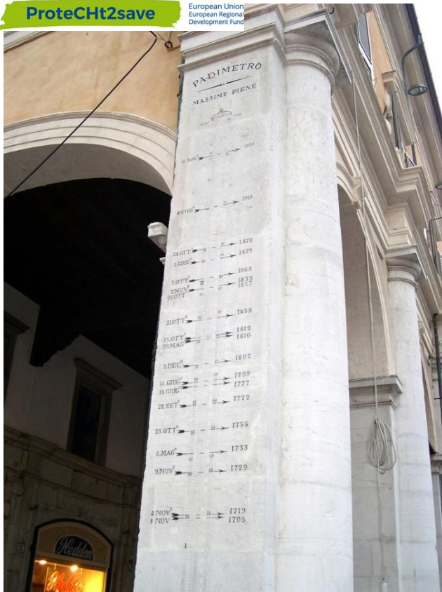
Figure 11. On the left: “Padimetro” of Ferrara. This monumental water gauge indicates the different heights and corresponding years of Po River level at Pontelagoscuro, a locality few kilometers distant from Ferrara city center. It is showed on a coloumn near the Cathedral square. On the right: the flooded area in front of Ferrara Cathedral.
