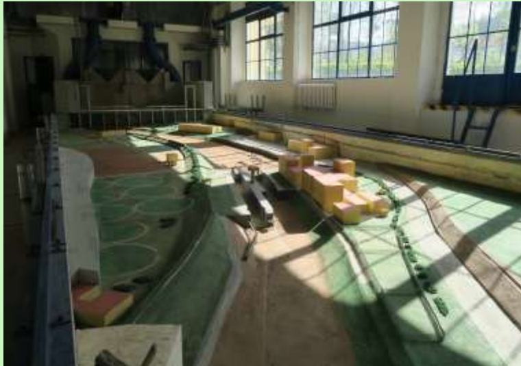
Physical model of river basin in Prague - Troja, CZ
