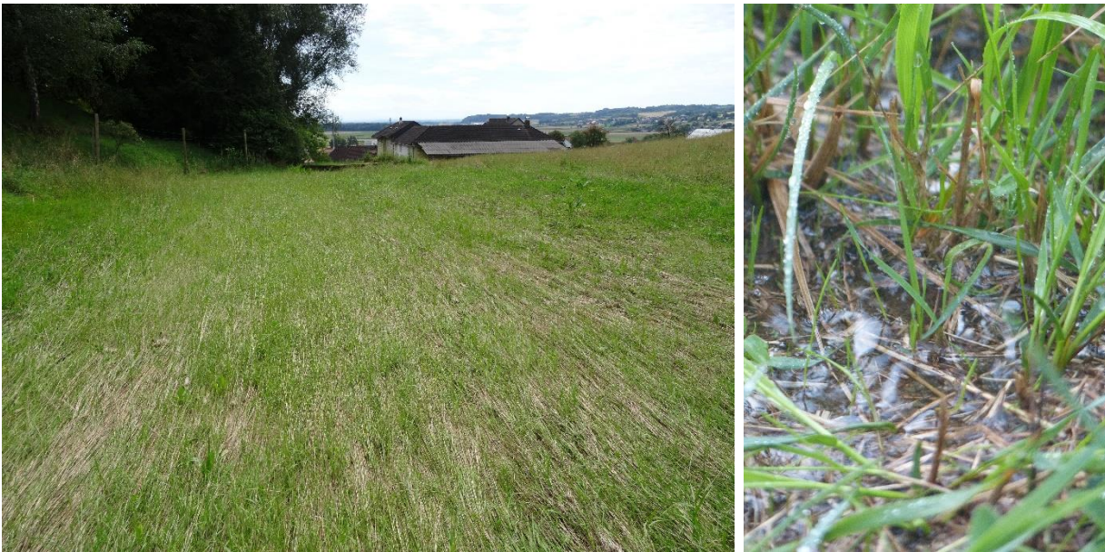
Figure 9: Vegetation laid down in the direction of flow after a pluvial flood in Schwertberg in 2016 (left) and runoff documented during an irrigation experiment (right). Depending on the water depth, the effective flow resistances here are higher (shallow water depth, right) or lower (vegetation laid down as a result of greater water depth, left) for the same land cover unit.
