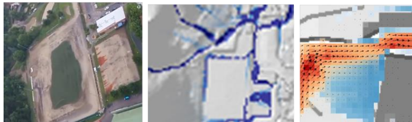
Representations of the contents of the three hazard mapping levels: from left to right: Observation with UAVs (level 1), flow pathway analysis (level 2) and hydrodynamic analysis (level 3); © Axel Sauer, IOER
