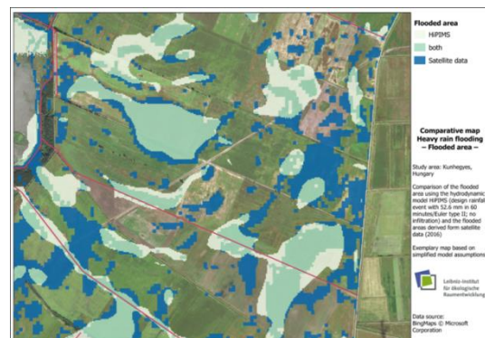
Hazard map based on a hydrodynamic simulation (level 3) for Kunhegyes, Hungary, and comparison with observed (satellite data) flooded areas.
