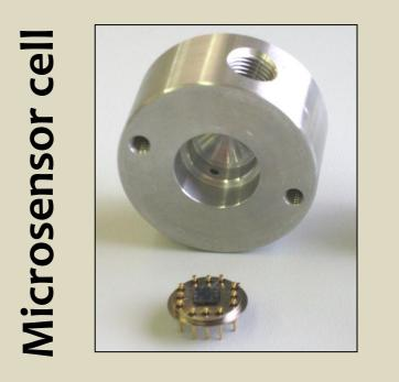
The chemiresistor conductance variations have been recorded in a **Gas Sensor Characterization System (Kenosistec)** upon exposure to different concentrations of NO<sub>2</sub>, keeping temperature and relative humidity constant in standard environmental conditions
