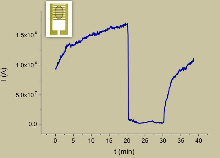
Dynamic response of **GTiO2** sensor to 1 ppm NO2 at room temperature
