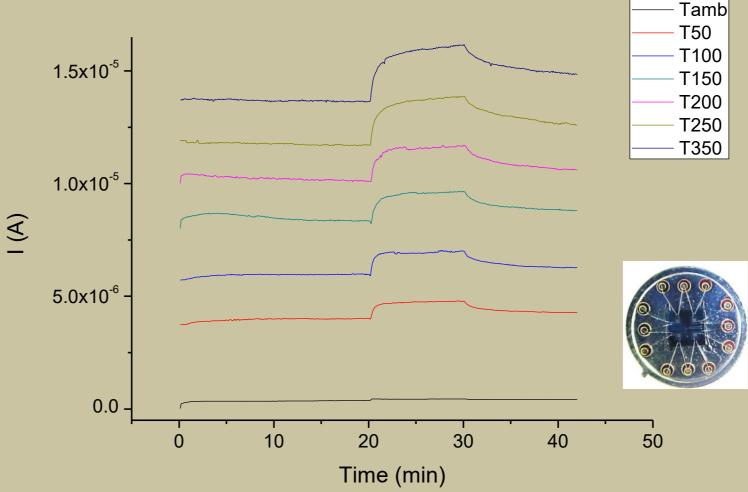
Dynamic response of the **GSnO2** device to 1 ppm NO2 in the whole temperature range Improvements of the responses were obtained for ZnO and TiO2 decorated materials at room temperature. In particular, device based on TiO2 decorated graphene shows a remarkable sensitivity gain towards NO2 gas.
