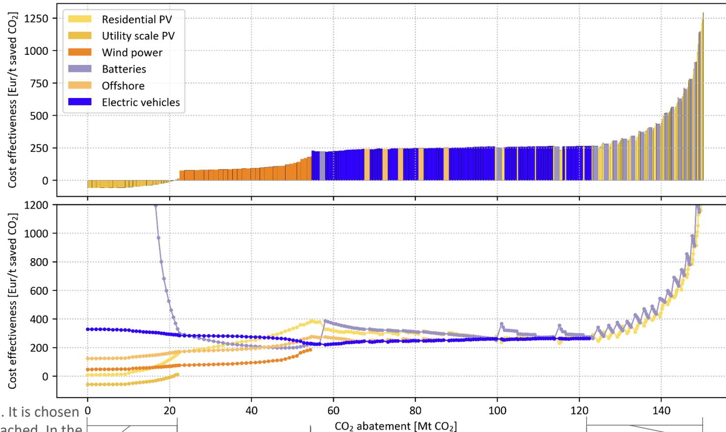
Utility scale PV has the lowest CE. It is chosen until the maximum potential is reached. In the meanwhile overgeneration is produced. CE from other generation sources increase. Residential PV CE increases with a similar trend due to the same shape of the generation profile
