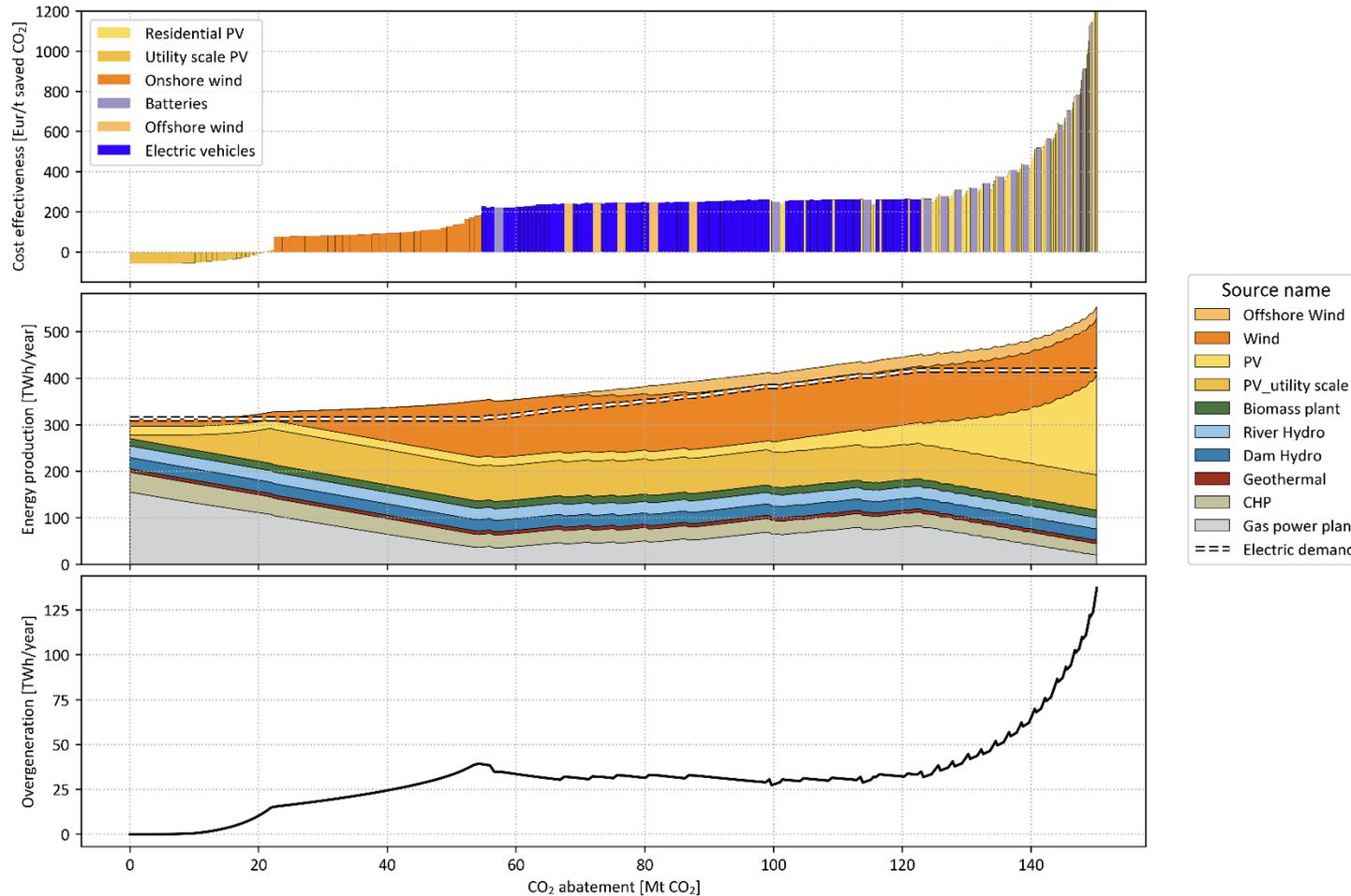
The RES uptake generates a growing overproduction that must be managed with grid stabilization measures
