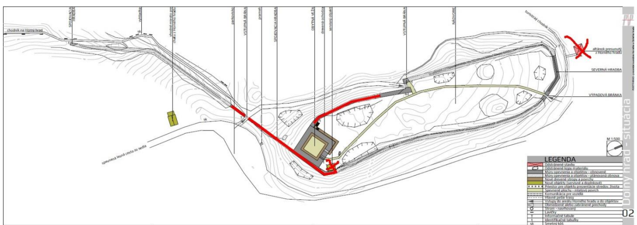
Figure 9 Ground plan from architectural study of restoration of the lower part of the Castle Pustý Hrad in Zvolen by Ing. arch. Miloš Pivko. Grey – already finished work, red outlined – planned work, x – denied building activities.
