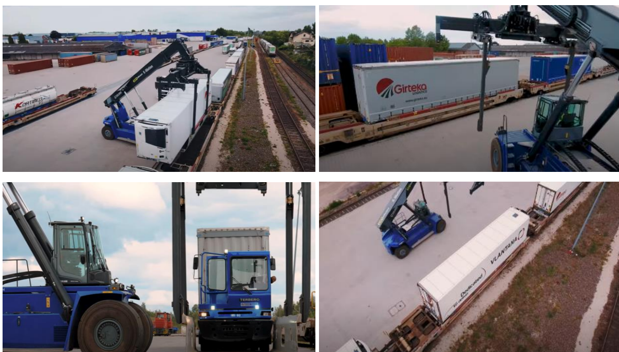
Figure 61: Semi-trailers being loaded onto the test train in Kaldenkirchen terminal
