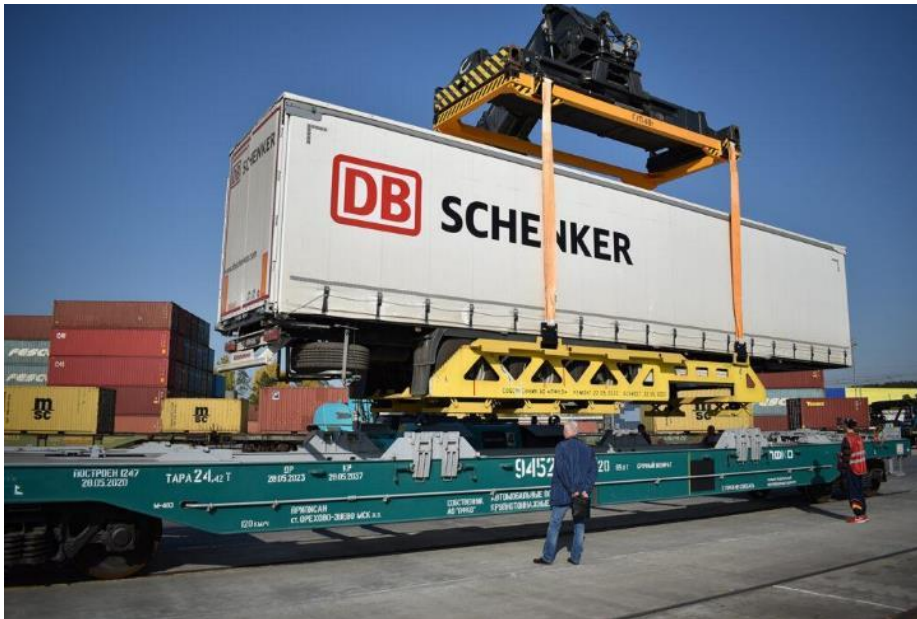
Figure 57: FFIFO wagon for semi-trailers in operation
