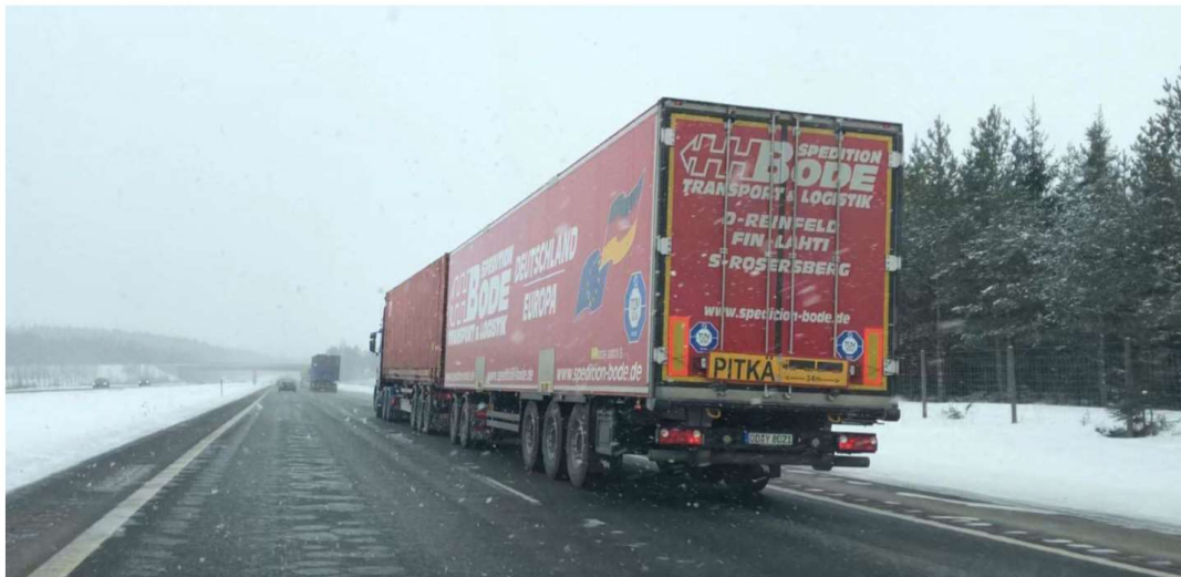
Figure 4. HCT trucks (34,5 m / 76 tons) have been a successful part of daily business for over two years in Finland. (Photo credit: Jukka Siren, Ramboll Finland)
