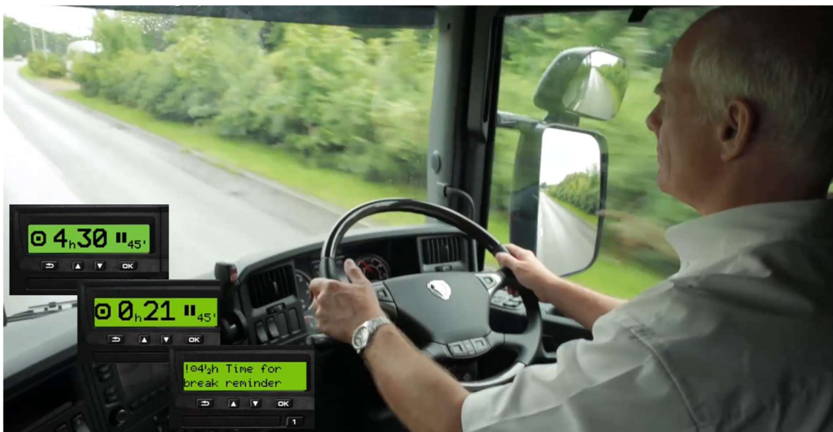
Figure 12. Tachograph follows the driving and resting periods. The basic rule is that you need a 45-minute rest after 4,5 hours driving. (Source: Scania video)
