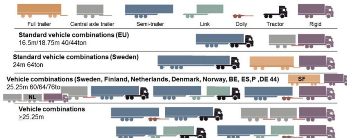
Figure 1 Standard and HCT-vehicle components and configurations
