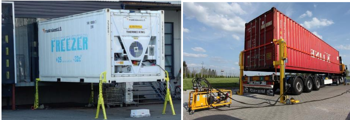
Figure 20. ConFoot (left) and Lifting Jacks (right)
