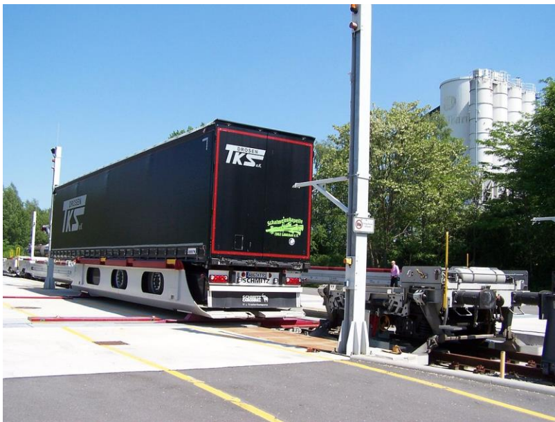
Figure 27. Loading station at the Cargobeamer terminal
