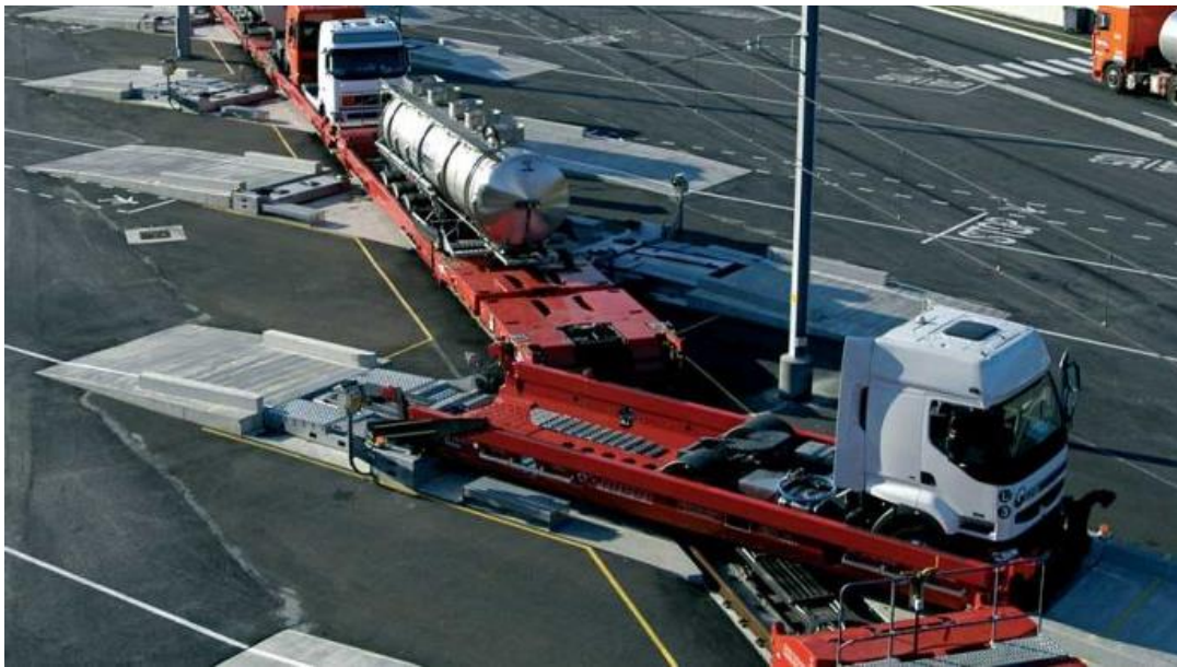
Figure 26. Loading station at the Modalohr terminal
