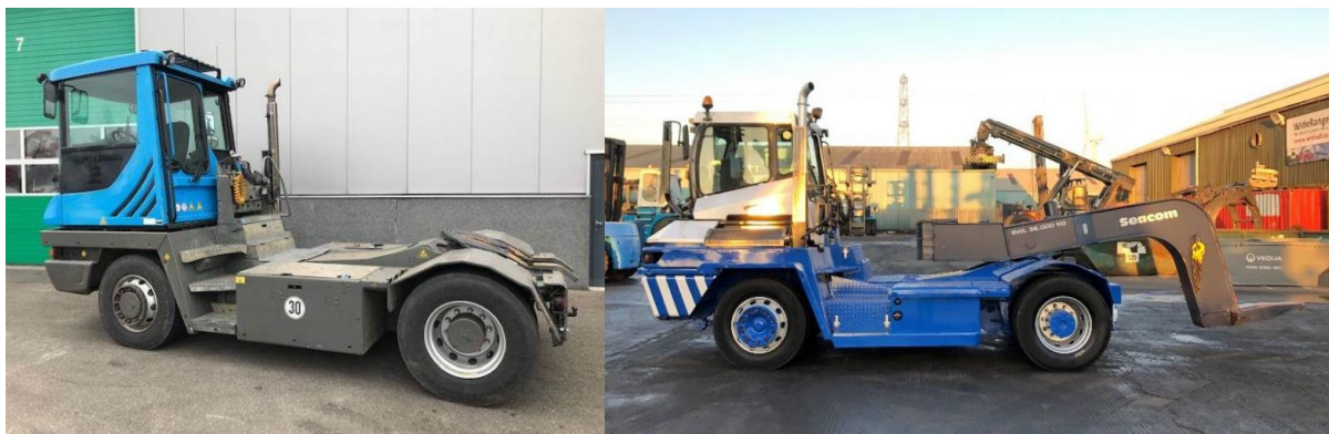
Figure 25. Terminal tractor (TT) to be coupled with terminal trailer (left) and roll-trailer (right) Source: tradus.com
