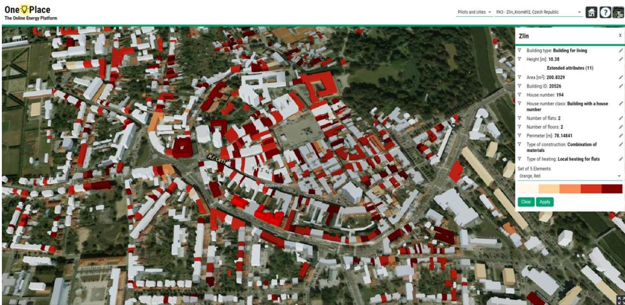
Figure 5: Example of aggregation functions within 3DEMS – energy sources used for buildings’heating. Source: OnePlace platform presentation
