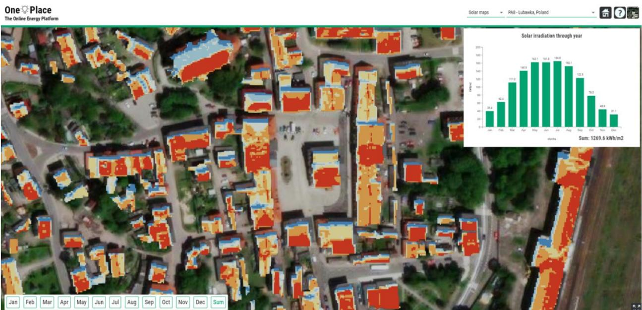
Figure 7: Example of web based visualization of photovoltaic PV maps. Source: OnePlace platform presentation
