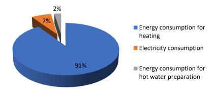
Figure 9: Energy consumption balance of the building for the PA2 – Sports hall.
