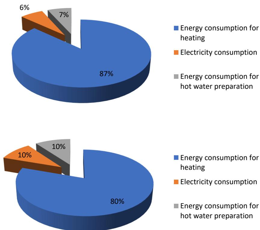
Figure 6: Energy consumption balance of the building for the PA3 – KROMERIZ basic school (before and after)
