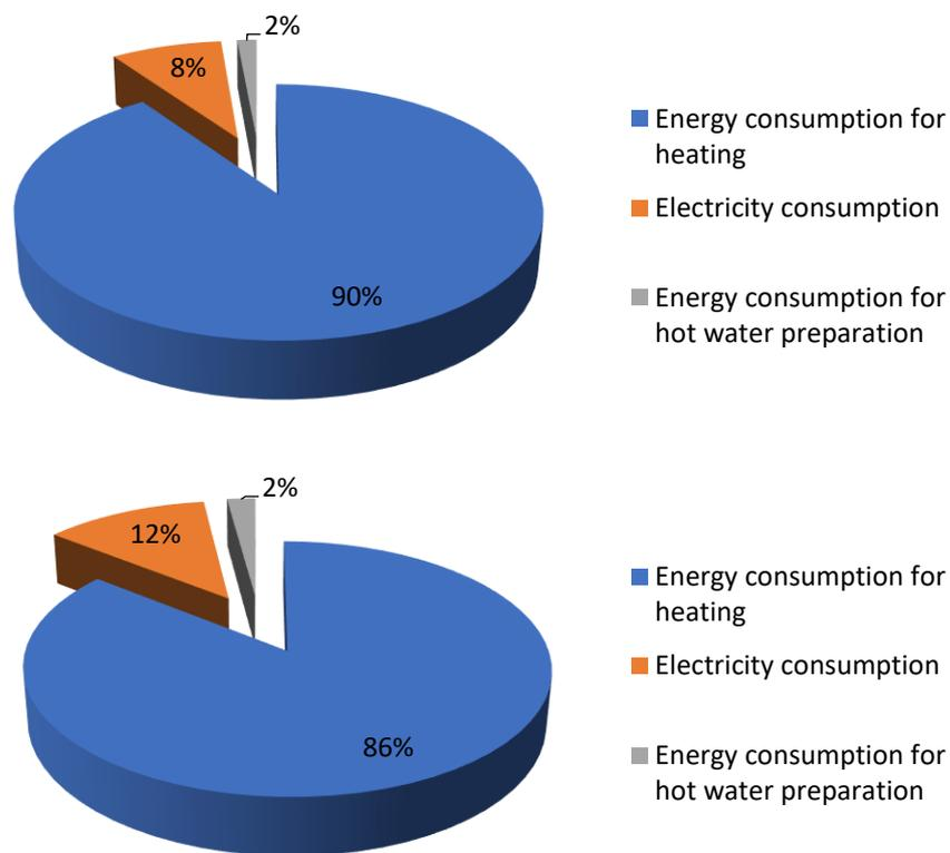
Figure 18: Energy consumption balance of the building for the PA3 – Pathology UH hospital (before and after)
