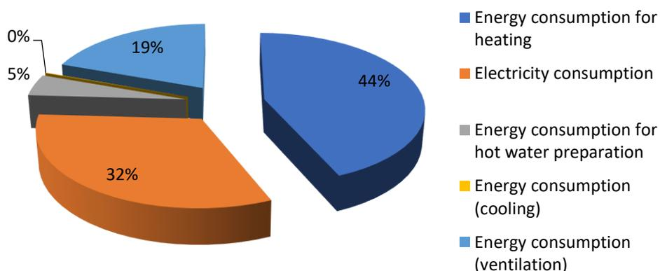
Figure 15: Energy consumption balance of the building for the PA3 – new intern medicine.
