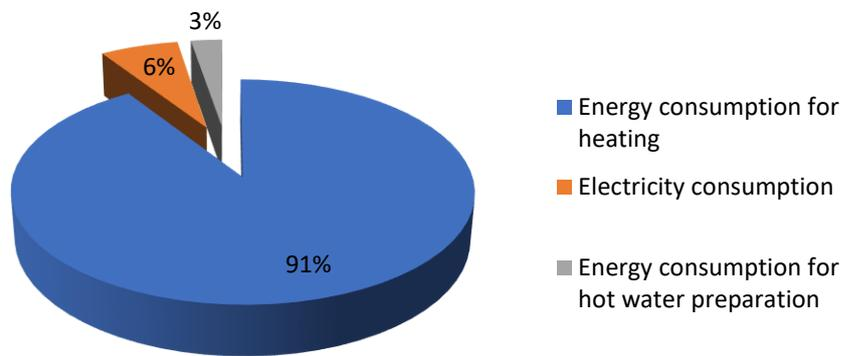
Figure 6: Energy consumption balance of the building for the PA2 – Primary School.
