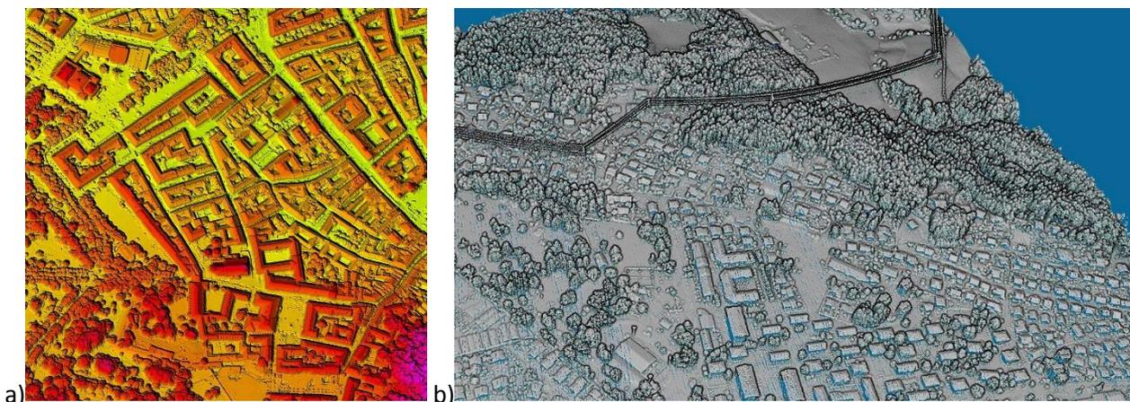
Figure 4: Example of photogrammetric point cloud derived from aerial images (a – source: FBK) and acquired with airborne laser scanning / LiDAR (b – source: Municipality of Velenje).
