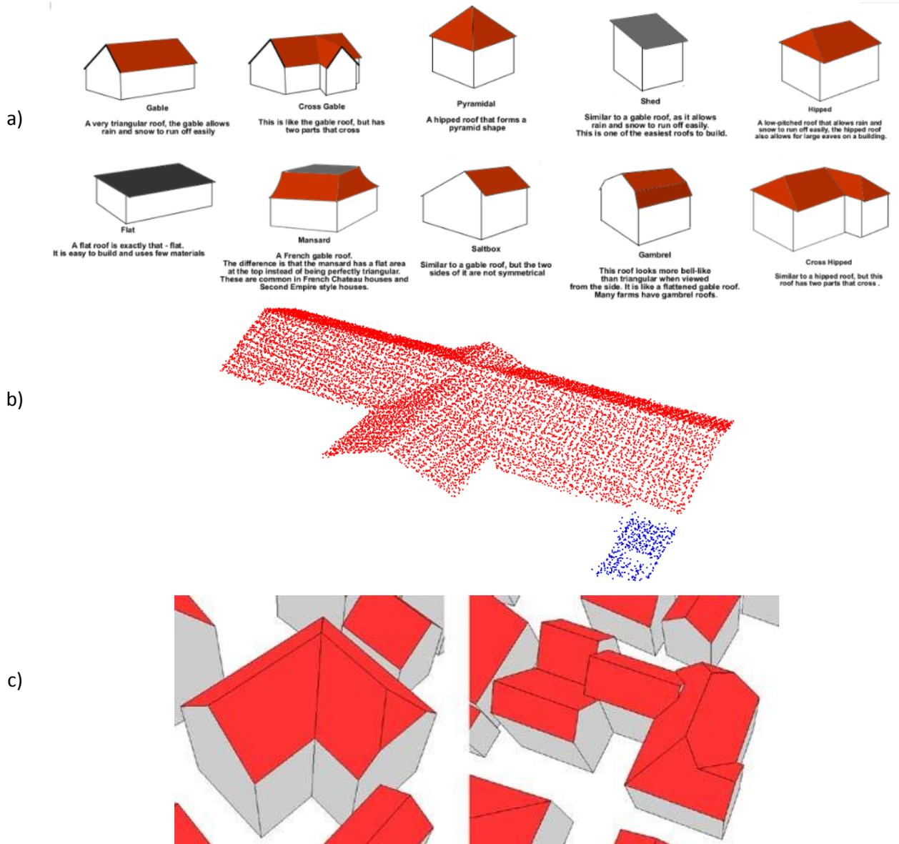
Figure 7: Example of roof primitives (a) which are then fitted onto roof point clouds (b) to derive LoD1 or LoD2 (c) building models (depending on the density of the point cloud and complexity of the roofs).
