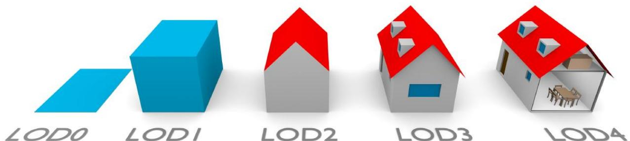
Figure 1: Different Level of Detail (LoD) in 3D building models (source: TU Delft).
