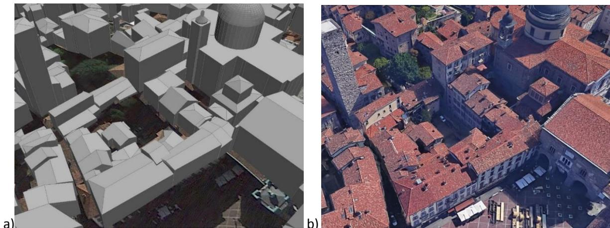
Figure 6: 3D building geometries (LoD2) derived fitting geometric primitives on point clouds (a: source: FBK) wrt polygonal mesh model (b: source Google Earth).
