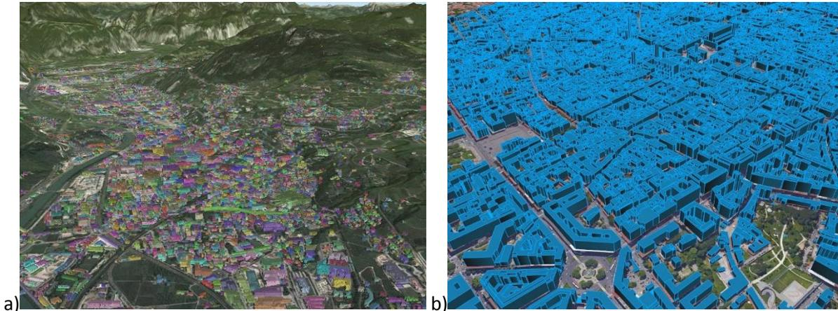
Figure 8: LoD1 over the city of Trento (a) and Bologna (b) generated extruding the available vector building footprint to a given height stored in the attributes of the vector data (source: FBK).
