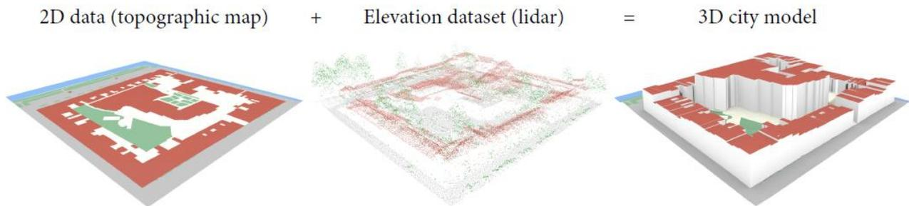
Figure 9: An hybrid approach to generate 3D building models: building polygons/footprints are extruded up to the height provided by a DSM (e.g. acquired with LiDAR)
