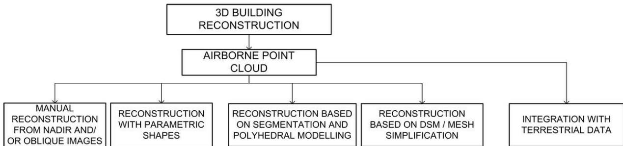
Figure 5: 3D building geometries from airborne point clouds: various methods to derive 3D geometries, e.g. through manual reconstruction, using parametric shapes, based on polyhedral modeling or applying a mesh simplification. Often terrestrial 3D data are also integrated.
