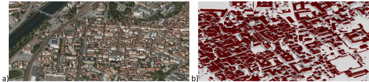
Figure 2: Different representation of a 3D city model: large and unique polygonal model with texture (a – source: FBK), single polygonal models in LOD2 (b – source: FBK).
