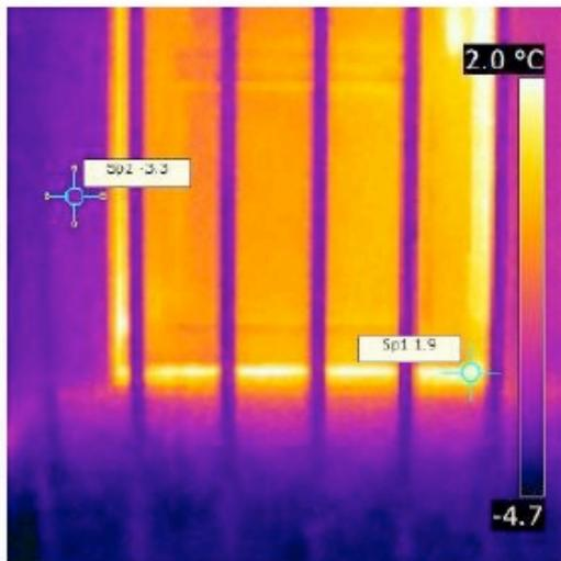
The thermal images show incorrectly adjusted exterior door leaf. In the upper and lower parts of the door an elevated temperature can be seen.
