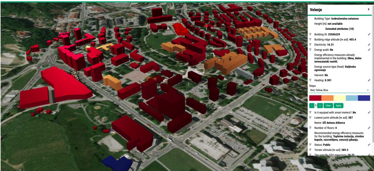
Figure 3: 3D buildings grouped and visualized based on their height (above) or heating needs (below).
