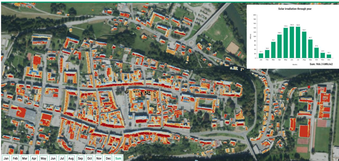
Figure 2: Photovoltaic (PV) potential of building roofs displayed per month and as a yearly sum.
