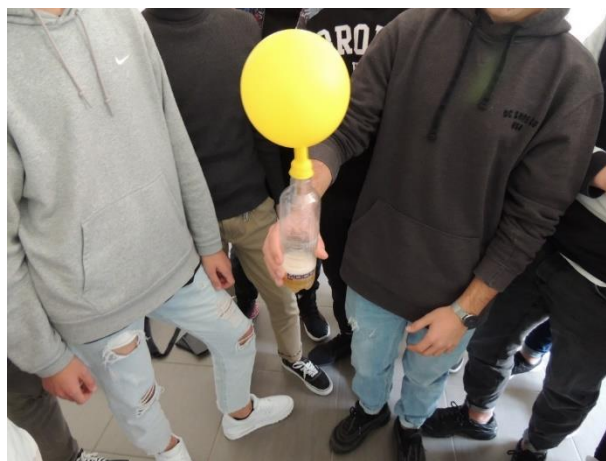
Figure 11. Experiment carried out in order to produce \text{CO}_2 adding vinegar to sodium bicarbonate.
