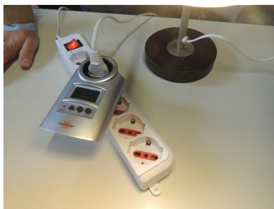
Figure 8. LCD Digital Energy Power Meter/Watt Voltage Calculator
