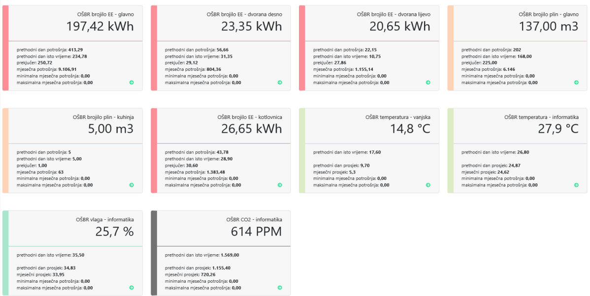
Figure 2: Central Monitoring System – Main dashboard. Source: REAN
