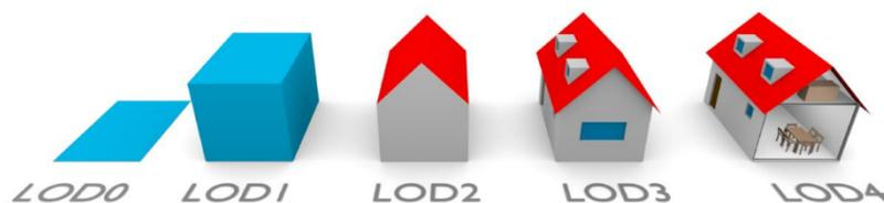
Figure 2. Different Level of Detail (LoD) in 3D building models (source: TU Delft).
