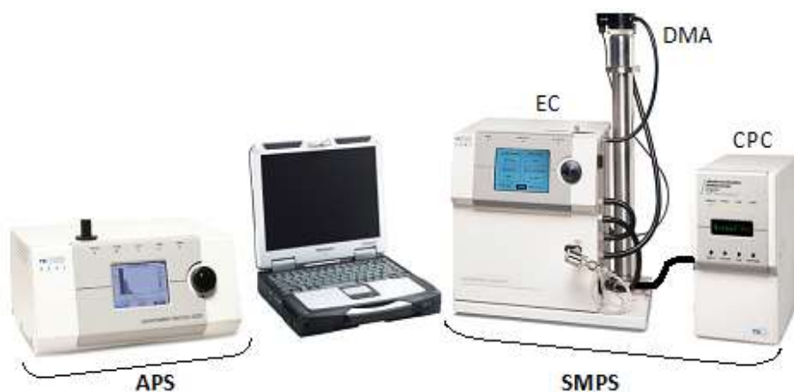
Rys. 5.20 Spektrometry Scanning Mobility Particle Sizer (SMPS) i Aerodynamic Particle Sizer (APS)
