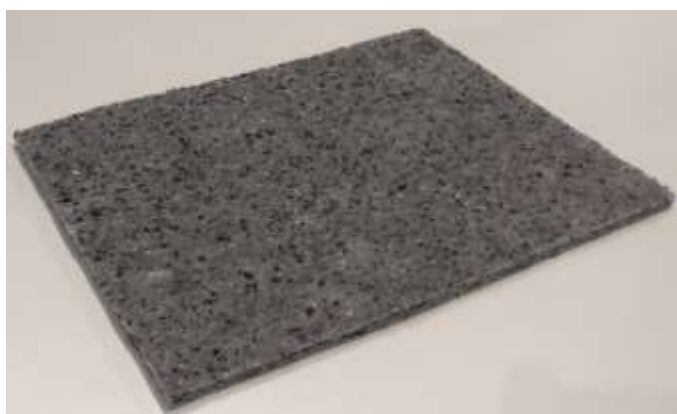
Photo 2 Recycled product - this is a nonwoven product achieved with airlay technology by using up to 85% of the waste shown in the picture above
