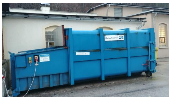
Fig.No.11: Mechanical press container for collecting of waste
