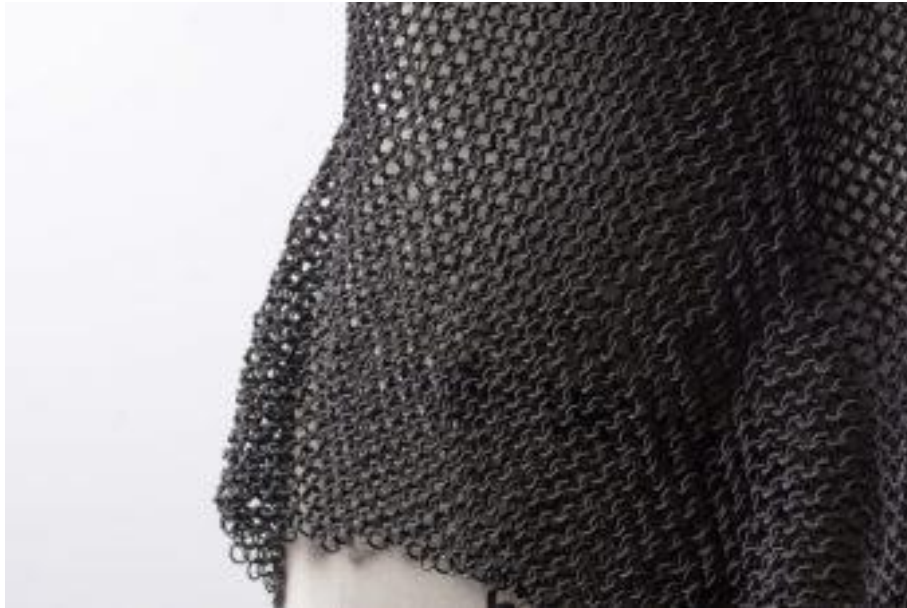
Printed suits of plastic with chain structure
