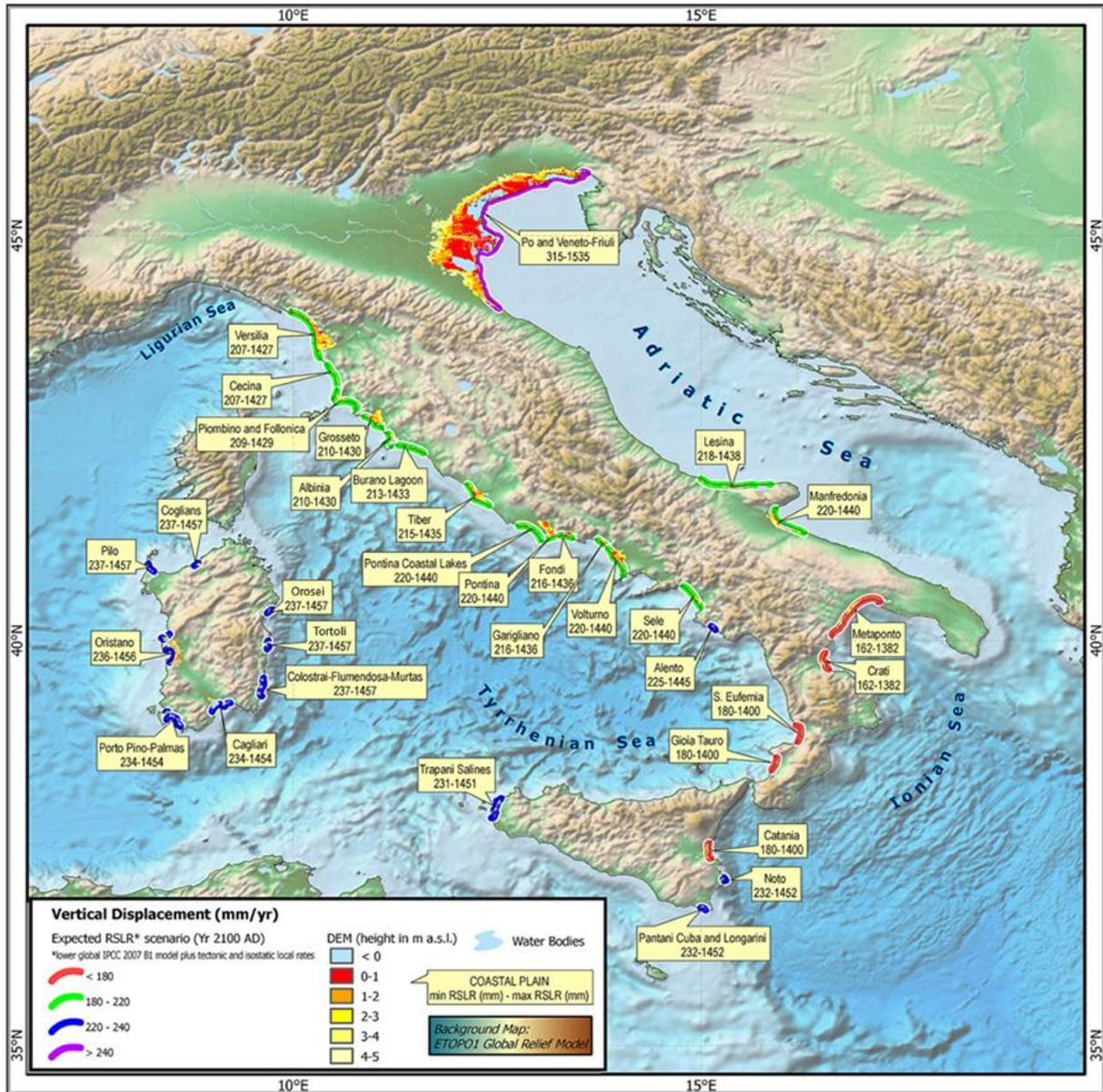
Figure 6: Italian coastal areas that could be flooded by sea-level rise in 2100 (Antonoli, 2016). Scenarios are based on the last IPCC report (Church et al., 2013) and Rahmstorf (2007) projections, high-resolution DTMs and rates of vertical land movements, including the glacio-hydro-isostatic model of Lambeck et al. (2011). For the Po Delta and Venice Plain, mean values are reported. Data do not include the contribution of local compaction and fluid (gas and water) extraction.
