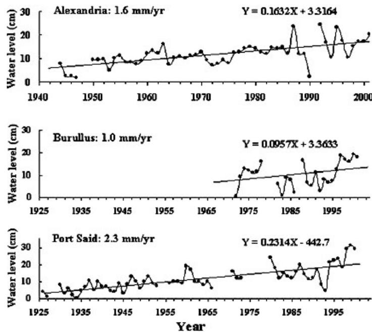
**Figure 25: Long term sea-level rise based on mean annual sea levels measured by tide gauges located at Alexandria, Burullus and Port Said (Frihy, 2003).**
