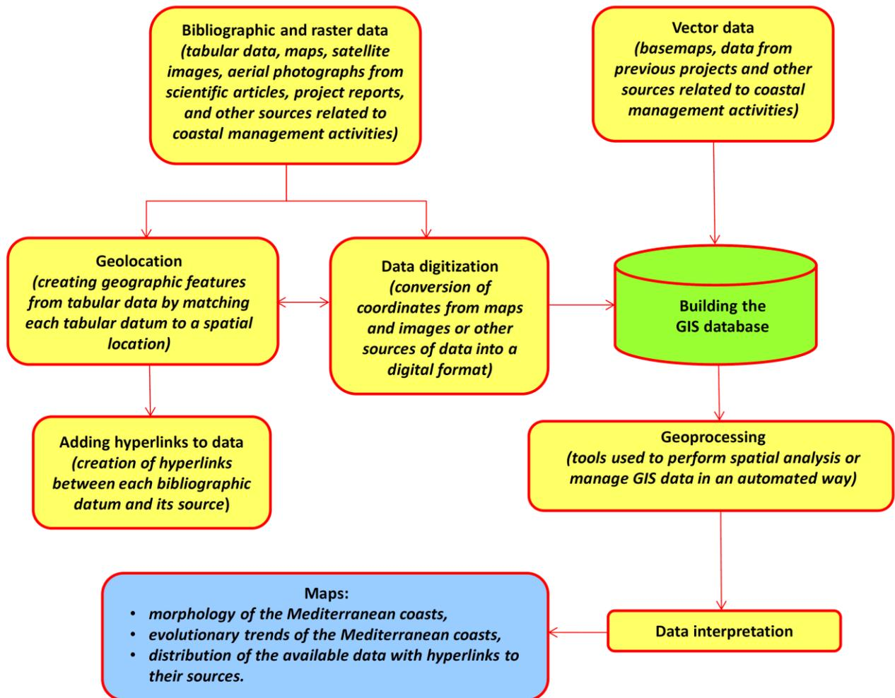
Figure 1: Block diagram of the GIS database.
