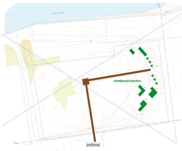
Fig 2. Situation of the area before the demolition of the decommitted bathing facility structures, and sketch of the designed intervention (SSI).
