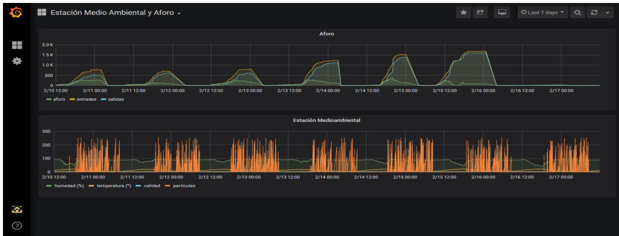
Figure 17. Platform's information screen with the measurements of the people counter and the air quality and meteorological variables.
