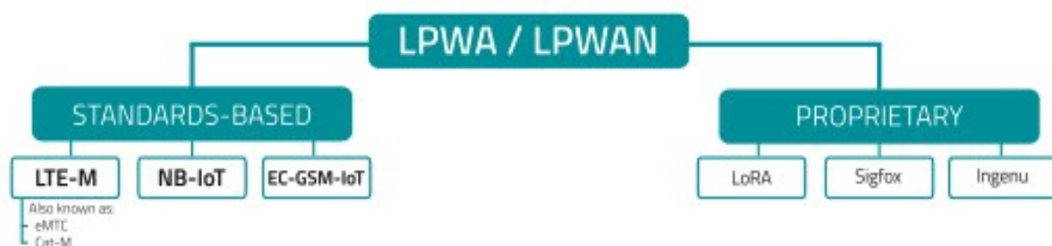
Figure 5: Categorization of LPWA/LPWAN communication technologies [6]
