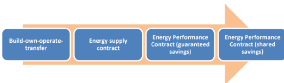
Figure 2 - Types of energy contracting according to increasing risk from left to right [2]
