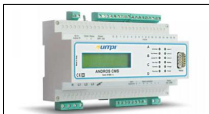
Figure 3.4: Andros CMS-CPU MODULE
