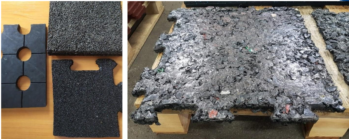
Fig. 3. Recycled “clean” granulate from preprocessed waste tires turned into products (left) and PLASTER Kuligowskiego® based on raw tire waste (right)
