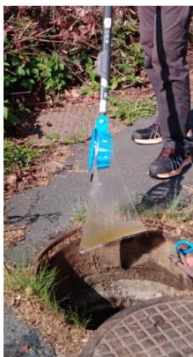
Figure 4. The fruit picker with the attached plastic bag. The plastic bag was inserted into the wastewater stream to collect samples.
