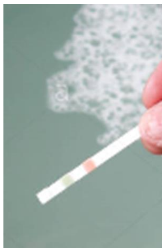
Figure 5. A quick analysis of the concentrations of ammonium and phosphate was carried out with test stripes.
