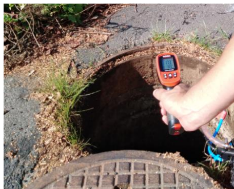
Figure 3. The temperature pistol was directed against the wastewater stream at the bottom of the well. The temperature was then shown in the display.
