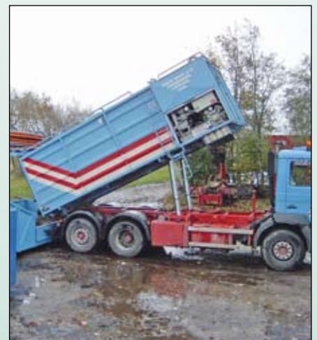
Once full the KSA is discharged by means of a hydraulically operated door on the dewatering chamber. The unit is then raised to allow the dewatered cake to slide out.
