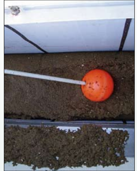
When the vacuum tank has been filled, the sludge is then pumped into the dewatering chamber via the machine room. During this process a polymer is added to cause flocculation. During and after the pumping process the dewatering takes place through the filter screens. The flocculated dry matter is effectively held back by special designed filter screens, allowing the permeate to drain into a collection chamber below.
