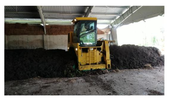
Picture 3. Mixing windrows during composting process
