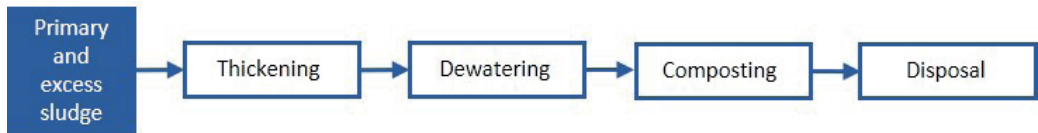
Fig. 1: Typical sludge processing model at small and medium WWT plants.
