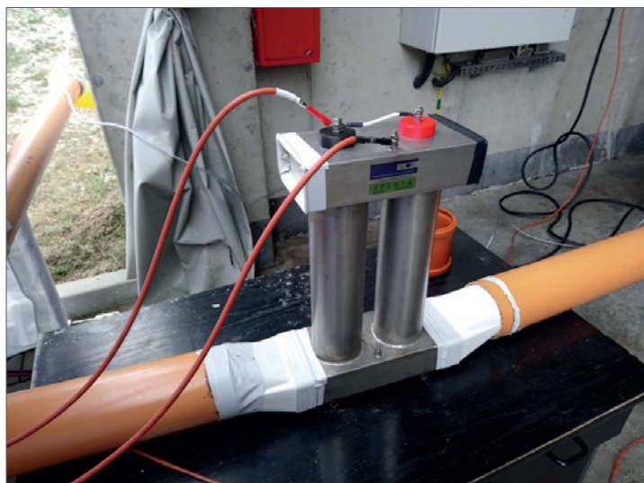
Fig. 4. Prototype of a single – tube corona discharge unit.
