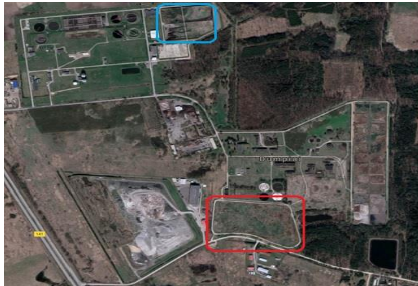
Figure 2. Orto-photo of the waste water plant „Klaipėdos Vanduo“ existing sludge storage sites: Red mark – old sludge storage site; Blue mark – existing 2 sludge storage sites.
