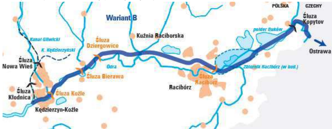
Fig. Odra-Danube connection (on the national part of the Koźle-Ostrava section) - variant B
